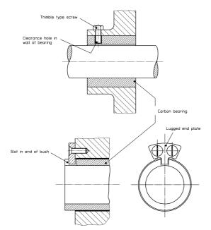
Sketch 8: Methods of retaining carbon bearings
