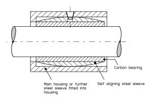
Sketch 2: Simple arrangement for self aligning bearings
