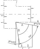
Top rake-Zero Clearance on faces A, B -10° Tool tip-Wimet 'N' or equivalent Speed 0.5 - 2.5 m/s Feed-Finish 0.125 mm per rev or less Cut-Finish 0.125 mm or less
