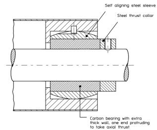
Sketch 3: An arrangement of self aligning carbon bearing for conveyor rollers, etc. illustrating provision for axial thrust taken on end face bearing
