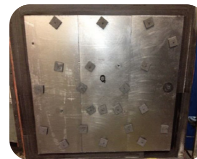
Furnace door with Graphite Foiled RGB after five Thermal Cycles to 1500 °C in Nitrogen
